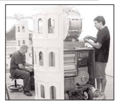
Treveris nearing completion as Don installs the pipe work and Dave attaches the bass drum beaters.
